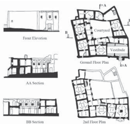
Fig. 5 House Plan of Djenne (on the left) Source: Oussouby SACKO (Seika University KIYO 39)
